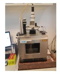
• Xtal Controller – for controlled crystalliation experiments Schubert et al., 2017
