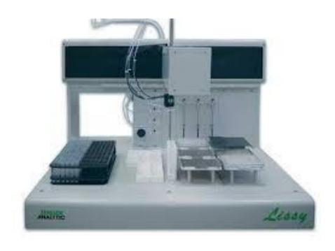
LISSY is modular state of the art *liquid* handler robotic system, combining sophisticated and flexible liquid handling with robotic manipulation. The modern, uncomplicated design integrates robotic and liquid handling functionality into a robotic arm, which glides on an x-rail to access racks modules on or off the workbench.
