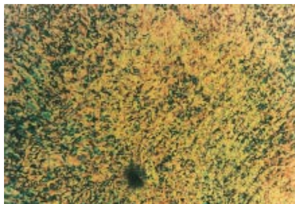
Fig. 3. Schlieren texture of the mobile cholesteric phase of 3d at 170 °C
