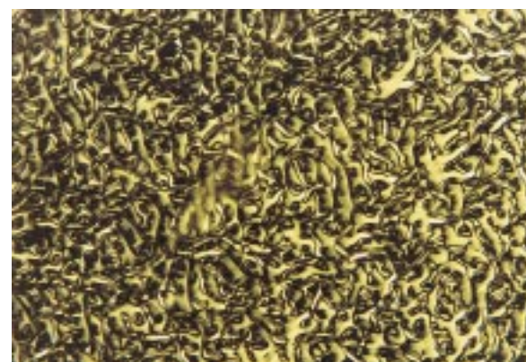
Fig. 5. Texture of the mobile cholesteric phase of 3b at 210 °C
