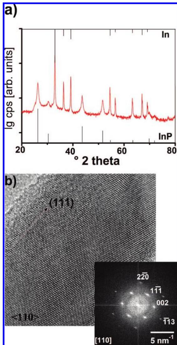
Figure 2. (a) XRD pattern of a In/InP needle sample (red), pure In (top), and pure InP (bottom); (b) HRTEM image of a InP needle in  $\langle 110 \rangle$  orientation with a growth direction along the (111) axis (arrow) and the FFT (inset) with the corresponding indexing.
