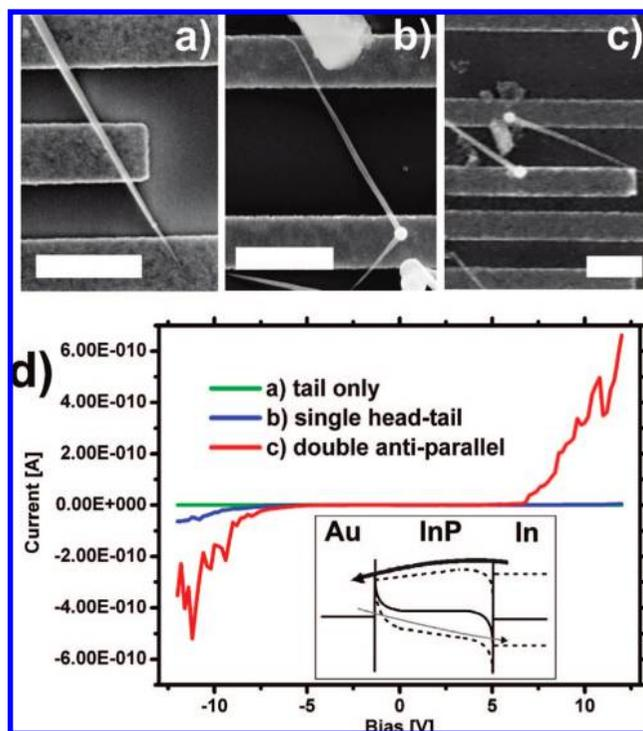
**Figure 3.** SEM micrographs of three different configurations of In/InP nanoneedles attached to gold leads: (a) only the InP tail bridges the leads, (b) a single nanoneedle attached with In head and InP tail, and (c) two needles attached in an antiparallel fashion (scale bar corresponds to 1  $\mu\text{m}$ ). The corresponding transport characteristics are shown in panel d. The inset shows the band alignment for the classical (thick arrow) and the tunnelling Schottky barrier.
