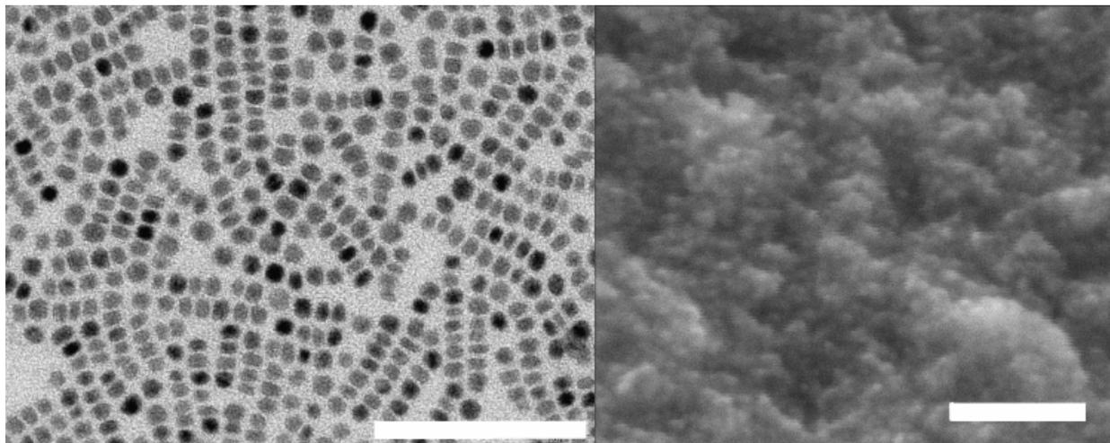
**Figure 1: Imaging of nanostructures.** (Left) TEM image of 1-dodecanethiol stabilized bismuth telluride nanoparticles on amorphous carbon substrate. (Right) SEM image of ligand-free, SPS compacted bismuth telluride nanoparticles. Scale bars correspond to 100 nm.
