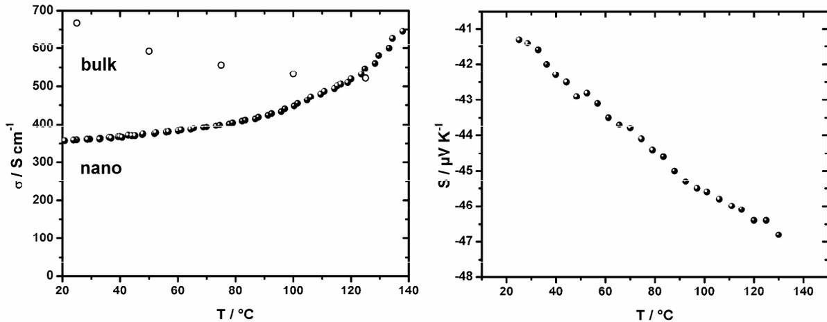
**Figure 2: Charge carrier transport. (Left)** Electric conductivity of nanostructured (full circles) versus bulk (open circles) bismuth telluride [13]. **(Right)** Thermopower of nanostructured bismuth telluride bulk solid.
