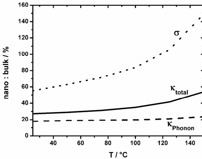
**Figure 4: Relative transport properties.** The effect of nanostructuring is investigated by plotting the ratio of electric conductivity (dotted), total thermal conductivity (solid) and lattice thermal conductivity (dashed) of nanostructured bismuth telluride divided by the values for bulk bismuth telluride [13] as a function of temperature.
