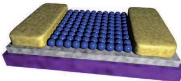
**Fig. 7:** Model of a super-crystalline monolayer of metal nanoparticles on gold electrodes.
