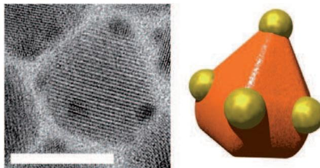
**Fig. 5: CdSe nanopryramid covered with gold clusters at the vertices (Left: Electron microscopy image, the scale bar corresponds to 10 nm; Right: Model of the structure).**
