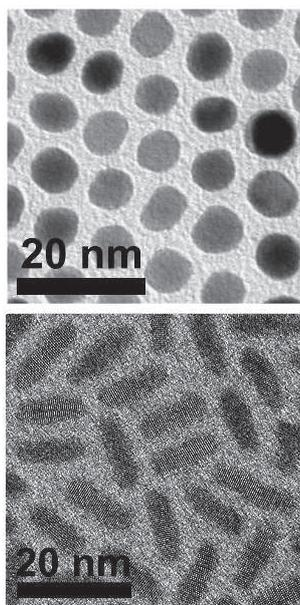
**Fig. 2: Nanoparticles of different nature and shape: (top) spherical CoPt nanoparticles, (bottom) rod-like CdSe nanoparticles.**
