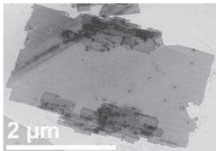
**Fig. 3: Electron micrograph of a single PbS nanosheet with a height of a few nanometers.**
