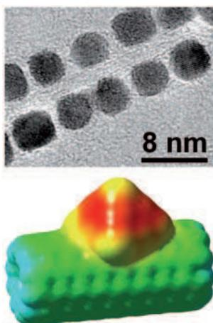
**Fig. 6:** CoPt nanoparticles attached to a carbon nanotube (top) and a representation of the electrostatic potential deduced from *ab initio* calculations (bottom). The metal cluster shows a negative potential (red) and the nanotube a positive one (green-blue). The attachment is a result of charge transfer and thus, an electrostatic interaction.
