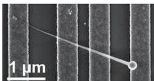
**Fig. 4: Gold electrodes (vertical bars) contact an InP nanoneedle with a spherical In head. The device works as ready-made Schottky diode and transistor.**
